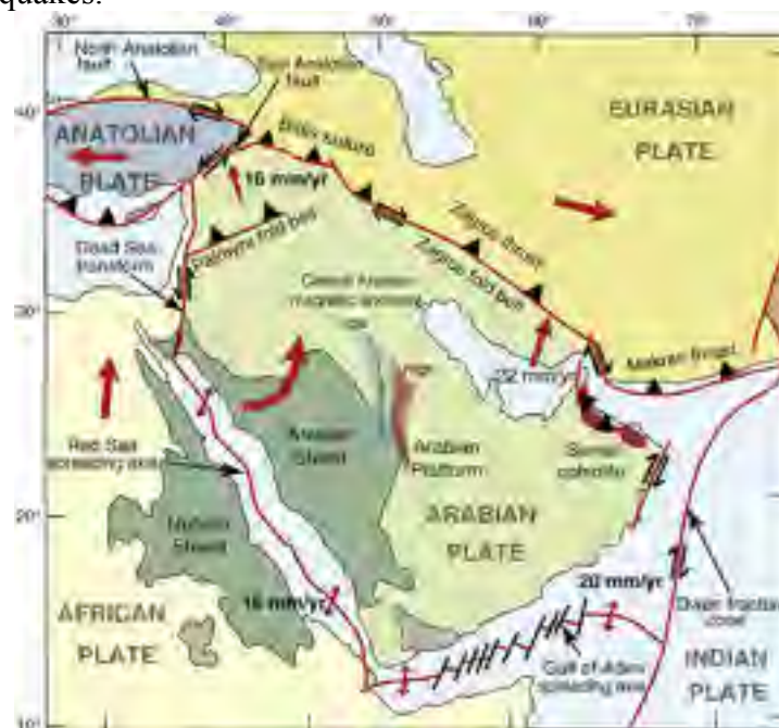
Fig. 8. Collision of the Arabian tectonic plate with the Anatolian plate resulting in Stress Transference and in its counterclockwise rotation.
