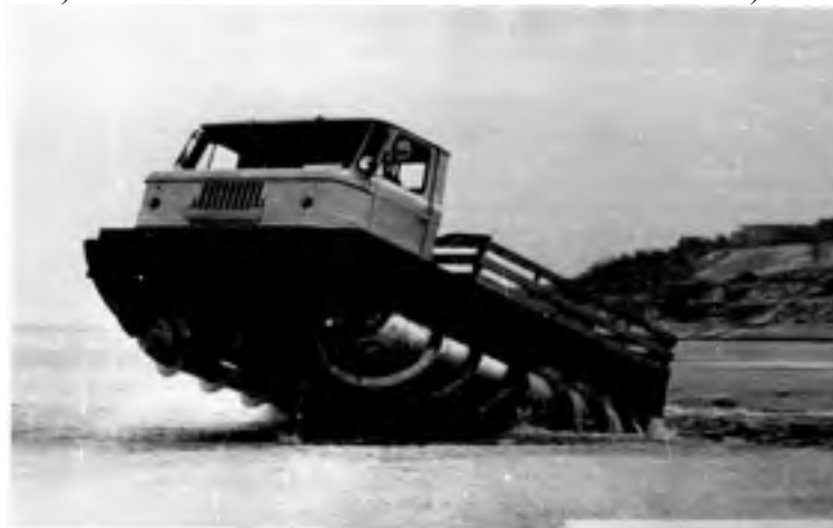
Fig. 7. Land - terrain machines with different types of propulsion: a - wheel; b - tracked; c - rotary-screw
