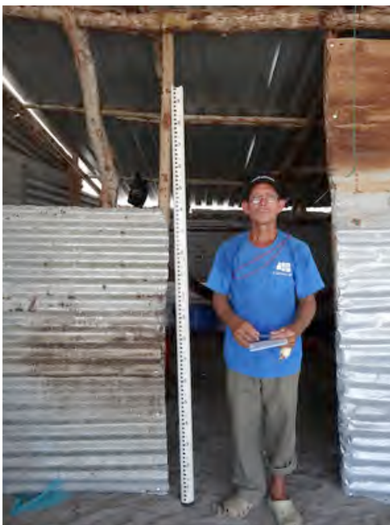
Figure 3.5 Jose Barrera-Garcia at the newly rebuilt ramada. Mr. Barrera-Garcia was swept away by the tsunami and suffered minor injuries. The tsunami flow depth at this location was reported by Mr. Barrera-Garcia to be over 2 m.
