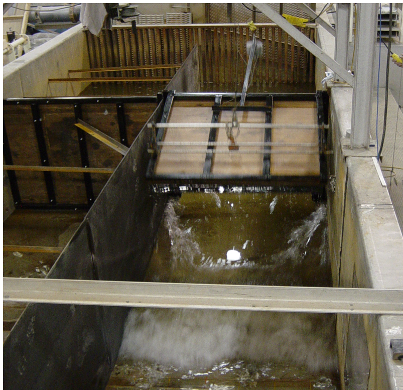
Figure 5. Turbulent hydraulic bore generated in the high discharge flume at the Canadian Hydraulics Centre
