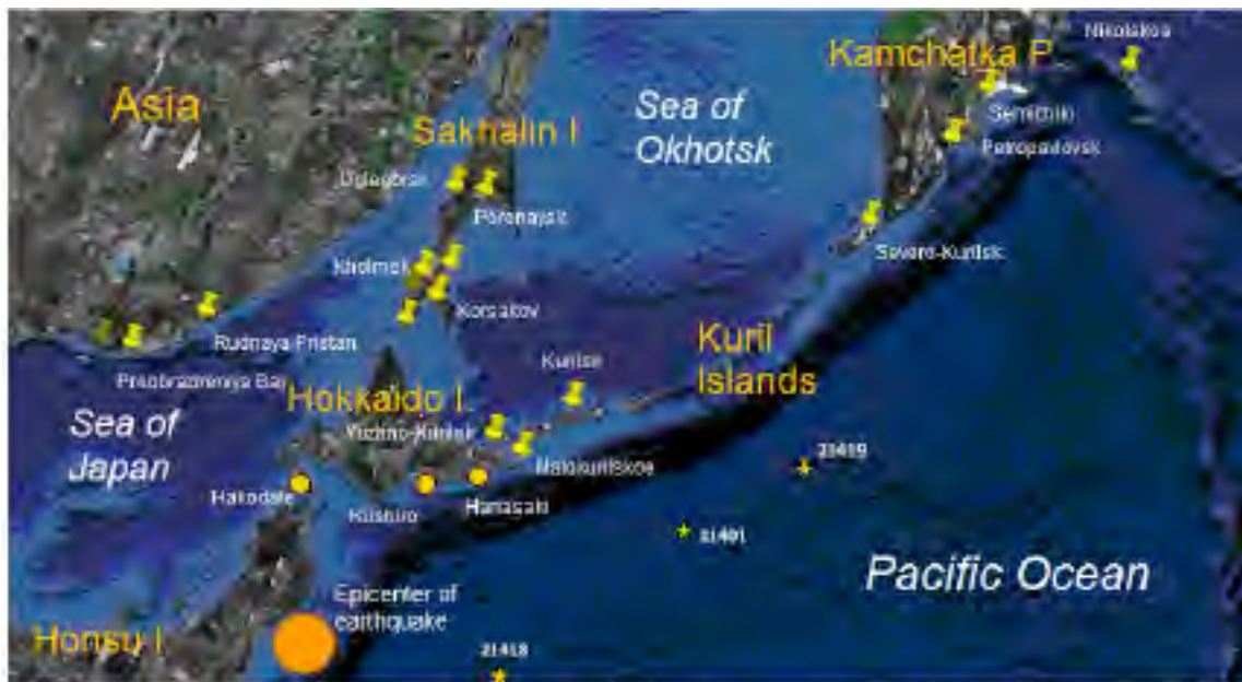
Fig. 1. Stations which recorded the Tohoku 11.03.2011 tsunami. DART stations marked by stars; coastal gauges of the Japanese Tsunami Warning Service marked by yellow circles and Russian TWS coastal telemetric gauges marked by yellow buttons. The earthquake epicenter of earthquake is marked by the orange circle.
