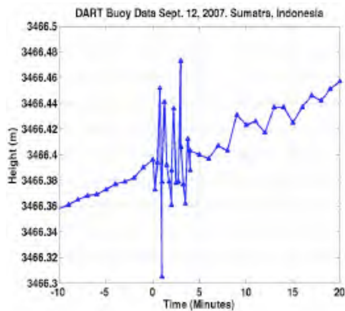
Figure 2. Pressure data recorded by a DART (r) buoy during the Sumatra tsunami event of Sept. 12, 2007. (Data from NOAA).
