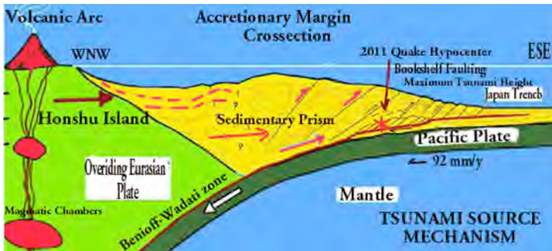
Fig. 12. Postulated Crosssection of the Accretionary Margin east of Honshu Island. Compression of the Sedimentary Prism and Subsequent Normal and Bookshelf Faulting contributed to the Tsunami's Source Mechanism and to greater Tsunamigenic Efficiency.
