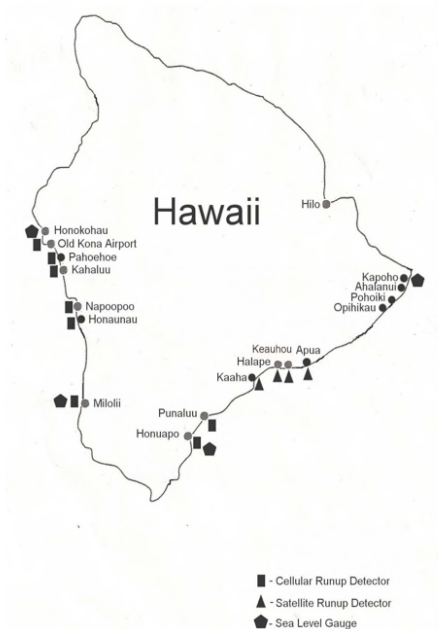
Figure 4. Site locations for Cellular Run-up Detectors (CRD's), Satellite Run-up Detectors (SRD's), and nearby Pacific Tsunami Warning Center sea level gauges.
