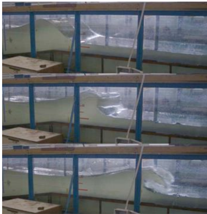
Figure 3 Formation of bore on slope beach (Nominal wave height = 80 mm)
