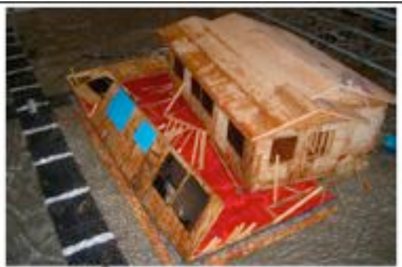
Figure 6. 1/6th scale residential structure that was tested to failure by wave impact.
