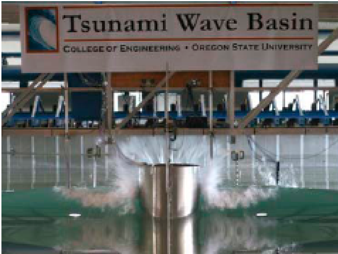
Figure 2. Tsunami wave impact on cylinders.
