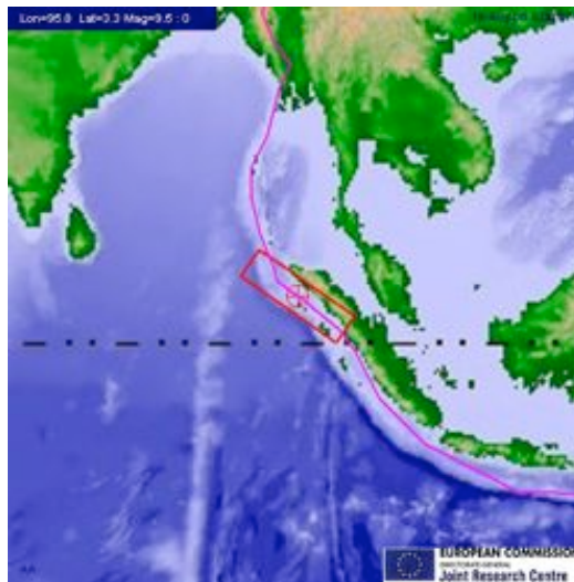
Fig. 5 - Creation of the fault direction and width
