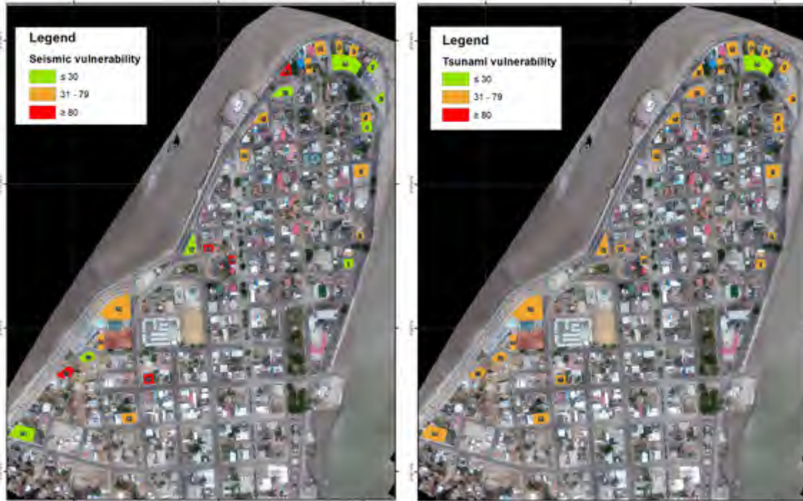
Fig.18. Maps representing the three categories assigned to seismic and tsunami vulnerability of the evaluated buildings. Green: Resistant structure with I_v \leq 30 ; Orange: Further evaluation is needed with 30 < I_v < 80 , and Red: Highly vulnerable structure with I_v \geq 80 .
