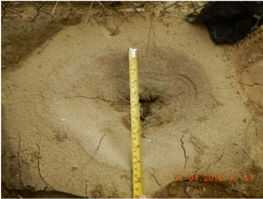
Fig. 22: Sand boils with a diameter of 30 to 55 cm. 585364mE 9913357mN. Intensity ESI = VIII.
