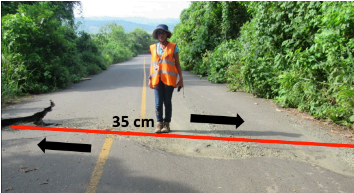
Fig. 18: Transcurrent displacement of ~35 cm on the paved road between San Vicente-San Isidro. Intensity ESI = VIII , coordinates (UTM: 573.419mE, 9.939.274mN).
