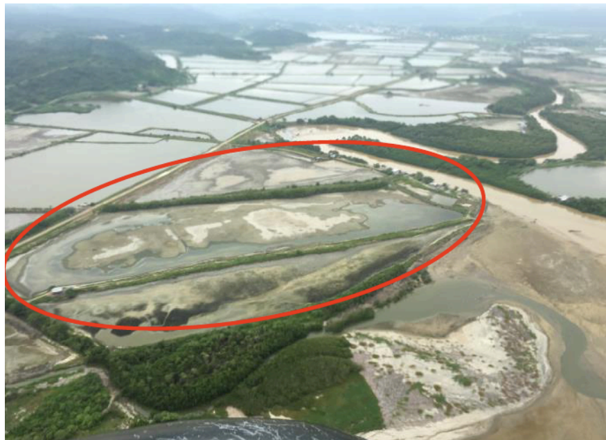
Fig. 12: Liquefaction evidence from GEER helicopter flyover of Manabí coast (Nikolaou et al., 2016), close to Jama ( 0^{\circ}12'31.7''S , 80^{\circ}15'22.5''W UTM coordinates 9976918.8N, 582762.5E).
