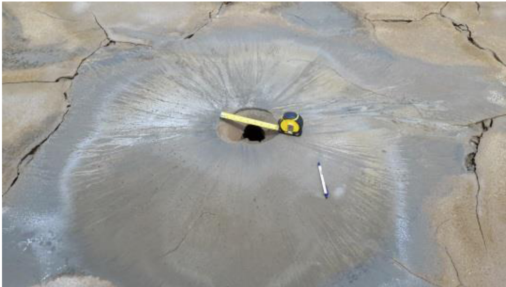
Fig. 23: Boca de Briceno Bridge liquefaction evidence in free-field and adjacent to embankment footing from GEER observations (Nikolaou et al., 2016) (GPS: 0°30'59"S, 80°26'31"W) UTM coordinates 9942920.8N, 562096.1E.
