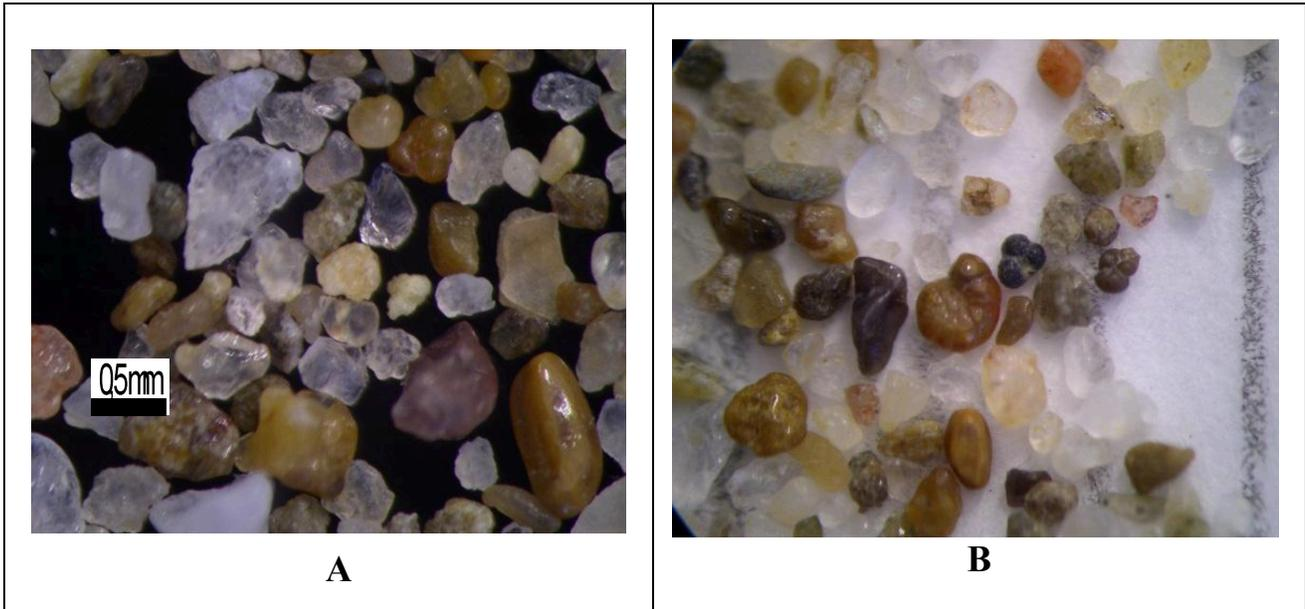
Figure 5. Optical microscope photographs of the shelly deposits of core CARLA-11.
