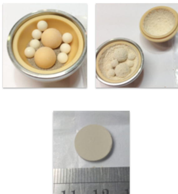
Fig. 3: sediment powder with grinding balls in a ZrO 2 bowl before (a) and after (b) grinding process, and after (c) pelletizing process.
