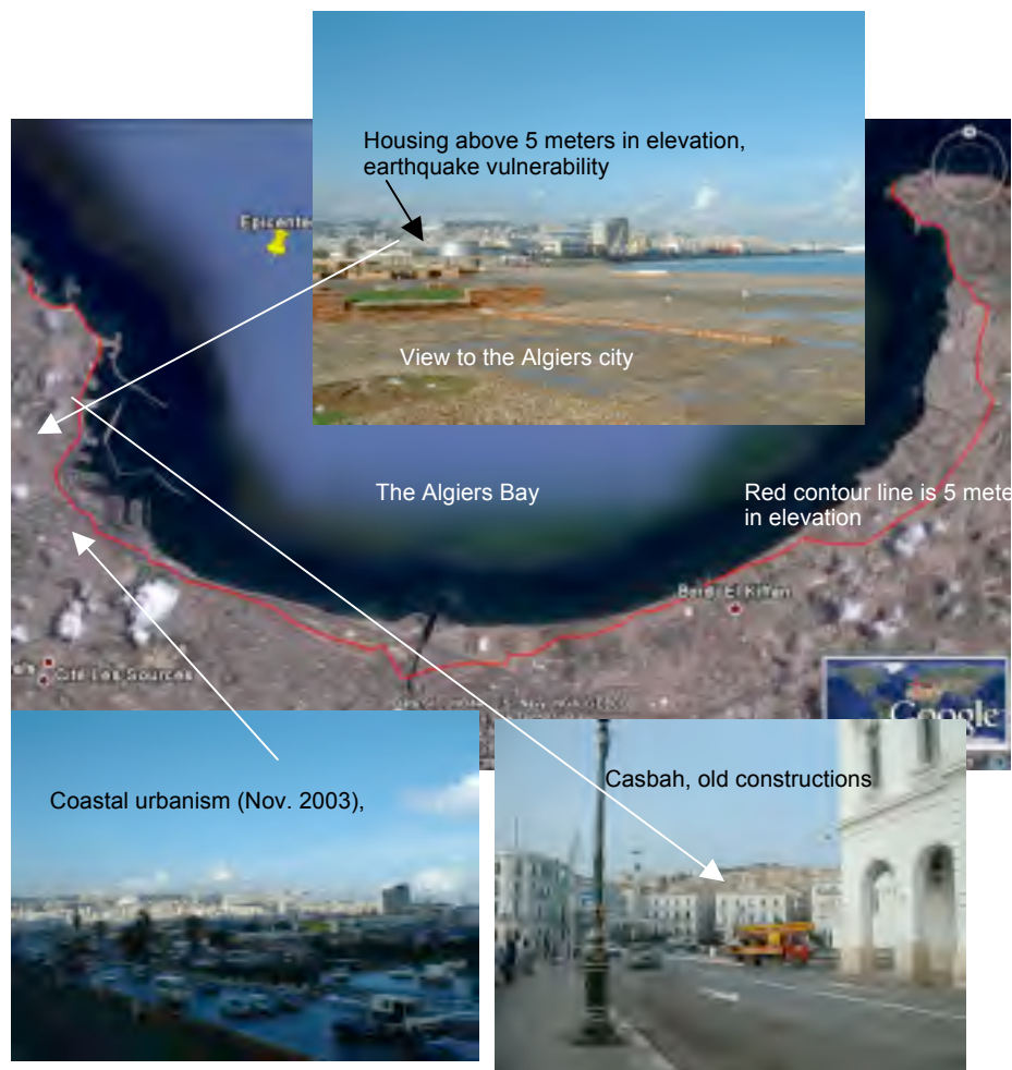
Fig. 7: Flooding map for Algiers region (with Google earth). The red contour line is 5 meters in elevation. Credit for Pictures: L. Amir
