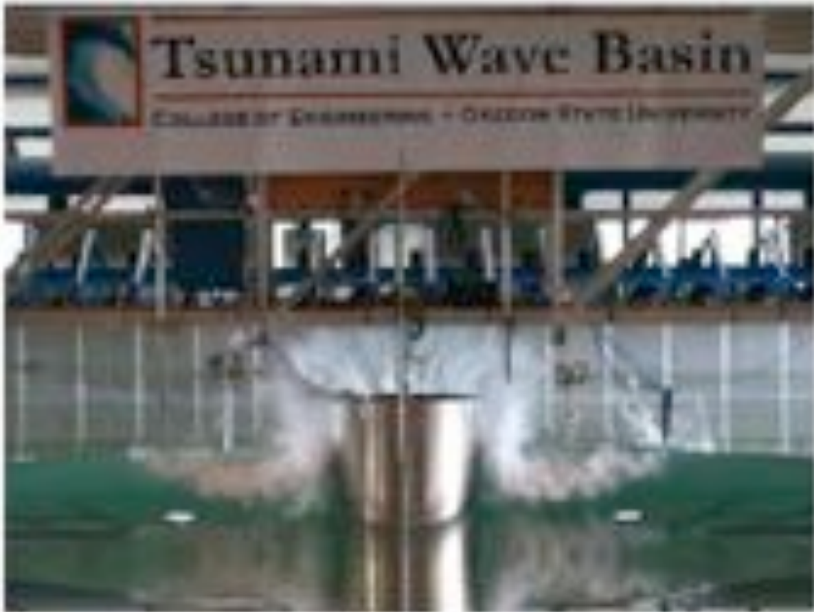
Figure 2. Tsunami wave impact on cylinders.
