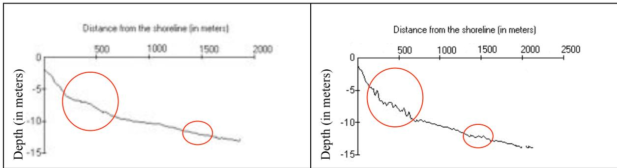
**Fig. 3 Profiles shows the areas of changes in the bathymetry (highlighted in the circles)**
